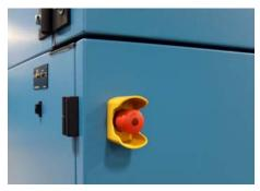
Immediately stop a test for any reason and save your product and chamber with the Emergency Stop button
