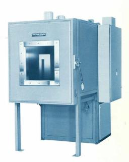
ambient and the test space. No tearing or deforming of shaker seal occurs as in chambers using sponge-type materials for sealing.
