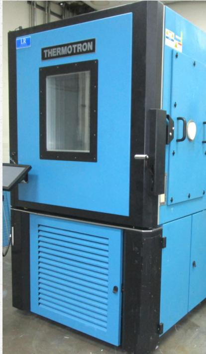
**NEW ARRIVAL – Thermotron Fast Ramp Temperature Humidity Climate Chamber Model #SE-600-15-15 with Temperature AND Humidity. I.D. of 40" X 26" X 34", Temperature Range of -70 to +180 Deg. C, and 10% to 98% Humidity.**
