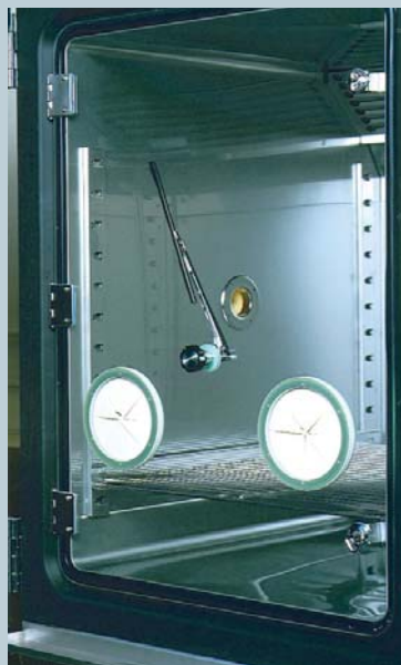
Includes hand ports to manipulate samples (14 cu. ft. size shown)
