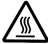
Danger!: High Temperature
