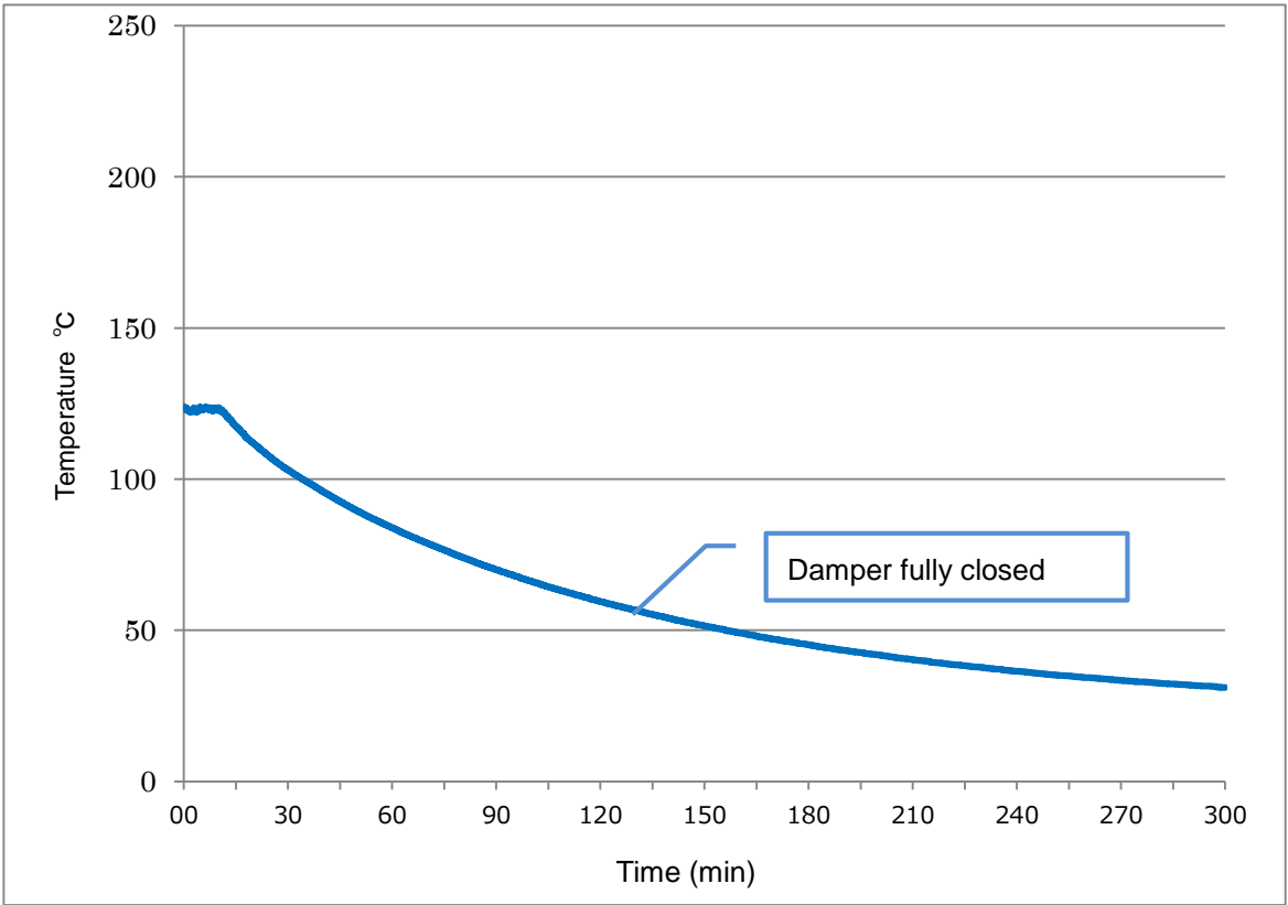
④ DNF301 temperature lowering curve (Natural convection)
