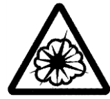
Danger!: Explosion Hazard
