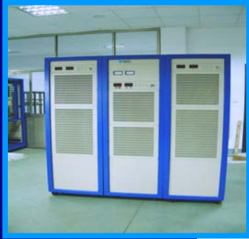
Our 120kva Replacement Amplifier for an Unholtz-Dickie T-1000
